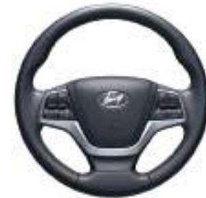
Steering wheel includes remote control functions for audio, cruise control and Bluetooth
